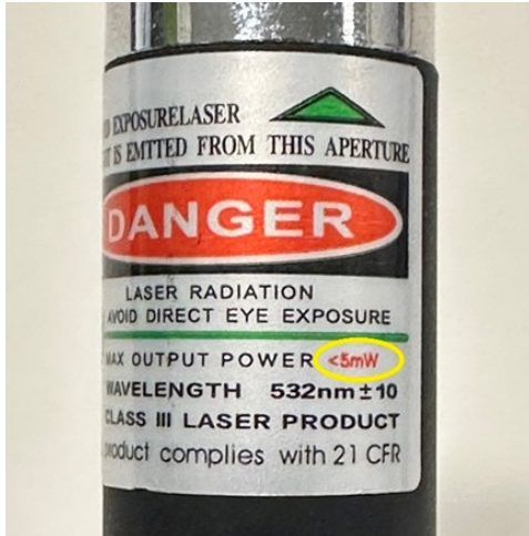
Fig. 3. Laser pointer labeled as < 5 mW output.
